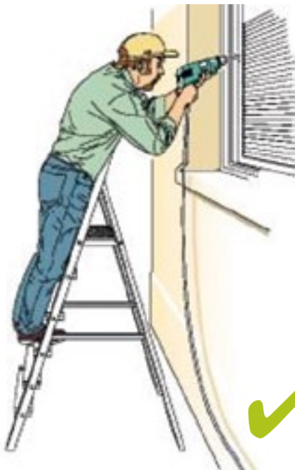
Figure 30: Correct – steps facing work activity.
