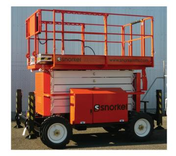
of working at height including when the ground is uneven. Like the other scissor models, (the S2770RT & the S3370RT) the S3970RT is a very versatile machine that can be operated on building sites or in warehouses and storage facilities. The operating costs are low and there is a wide range of options and configurations available for this machine.
